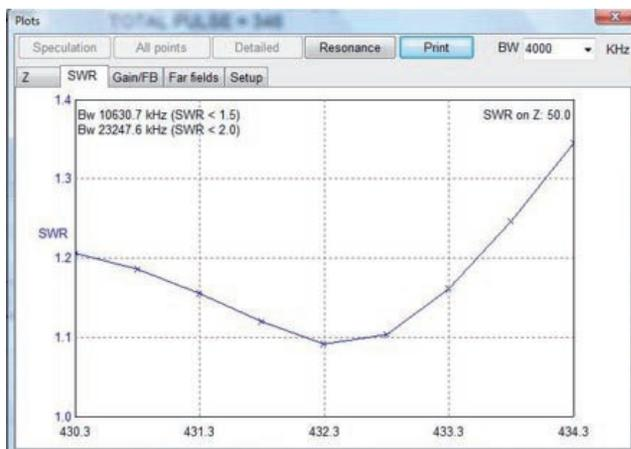
Fig. 2 - 31 el. 432; SWR vs frequenza
